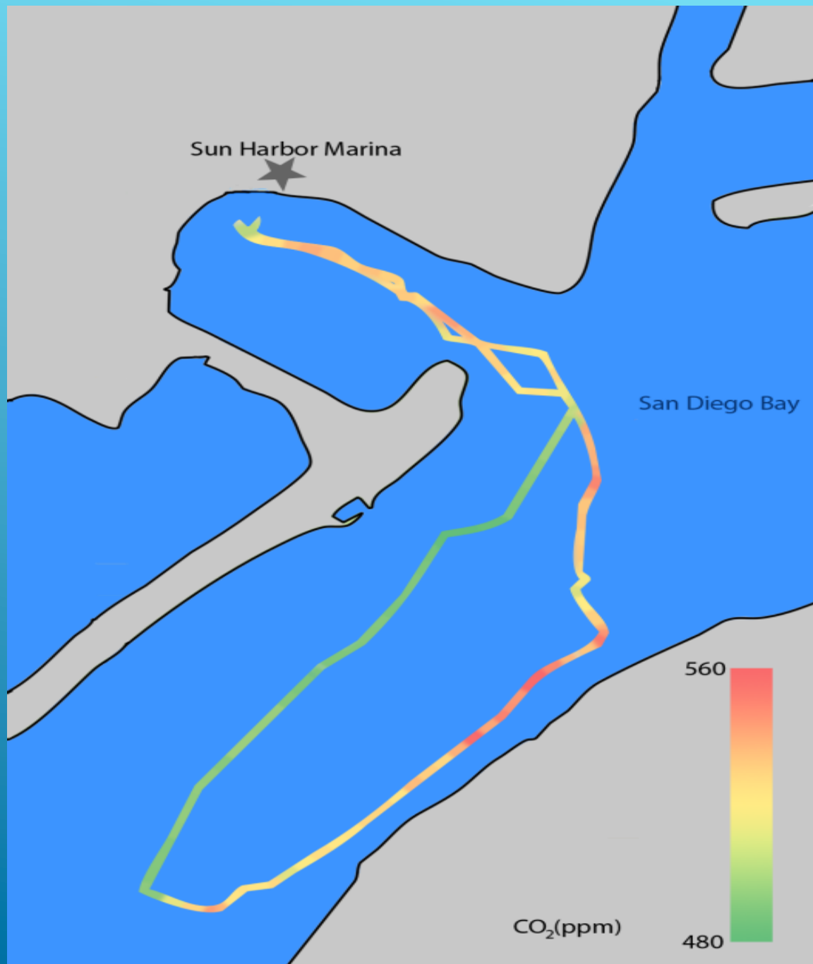
Figure Sampling path across San Diego Bay and the CO 2 concentrations measured
